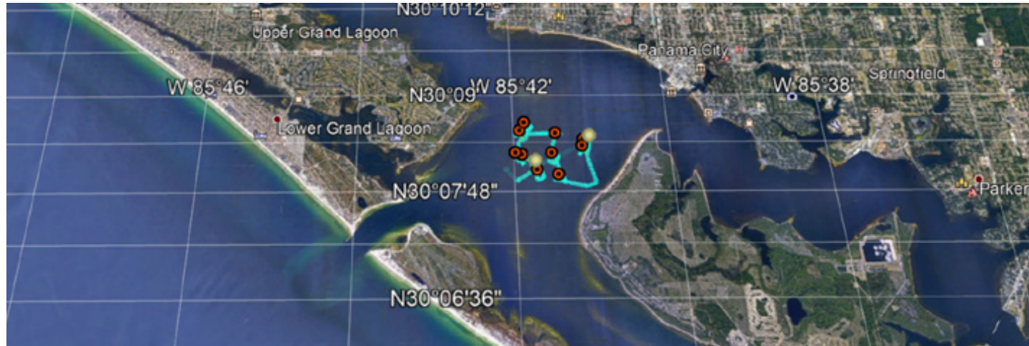
Bird-eye view of the sea tests in Saint Andrew Bay in Panama City, Florida. The red dots show the locations of targets to be identified and the green lines show the pathway taken by the autonomous underwater vehicle, using algorithms developed by Cornell and the U.S. Navy.
